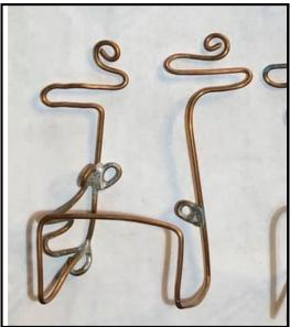
**Specimen hangers** are made of bent, 12-gauge electrical wire. Philip's mother designed the hangers.
