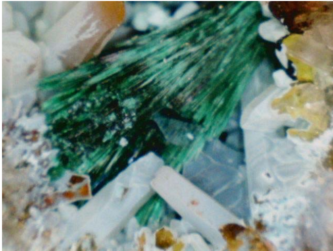
Monarch mine vug with malachite needles and azurite-covered quartz viewed at 30X
