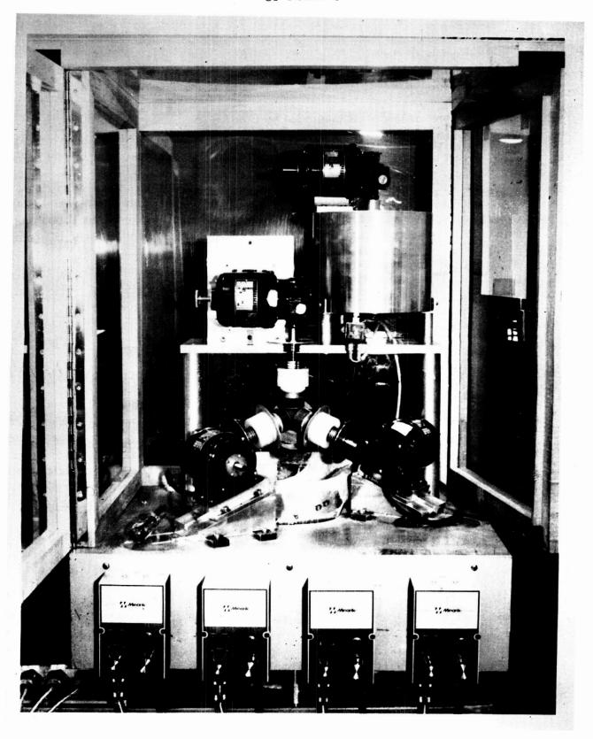
Figure 6. Polishing machine with enclosure.
