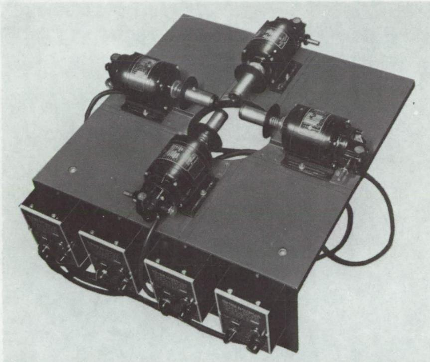
The machine shown in the figure will finish a ball to roundness (sphericity) within 12.5 nm (half a microinch) from any type of hard material. Machines used previously would produce a ball with accuracy of only 125 nm (five microinches) roundness. Grinding and polishing of the ball to this tolerance are accomplished by lapping elements on four to six motor-driven spindles.
